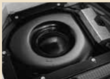
50-litre 'marshmallow' tank located in spare wheel well on Astravan. Please note the floor height is 90mm higher compared to the standard vehicle.
